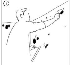
Prepare the surface: fill in the holes. Remove the socket covers and switches.
