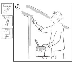
The sensitive parts of the wall need to be glued: wall, door frame/top and bottom edges.
