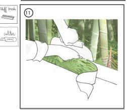
Cut off the excess with a cutter using the spatula (be sure to use a new blade).
