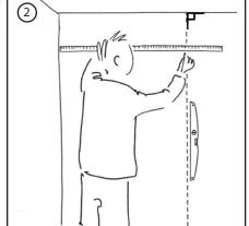
Measure the width of the first strip. Use a level to draw the dotted lines.
